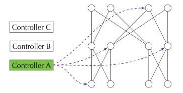
Controller install/remove flow-based routes at routers
