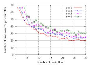
*r* = redundancy factor Redundancy is almost free
